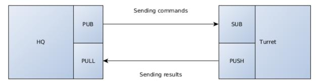
So as you can see this is pretty simple, the HQ send orders to the turrets using a PUB/SUB pattern, and the turrets will send results to the master using a PUSH/PULL pattern.
